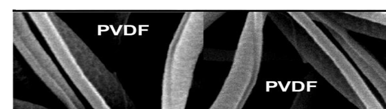
HRSEM image showed the same tendency to form strip shaped nanofibers as for PAN membranes and also the same formation of hollow fibers
