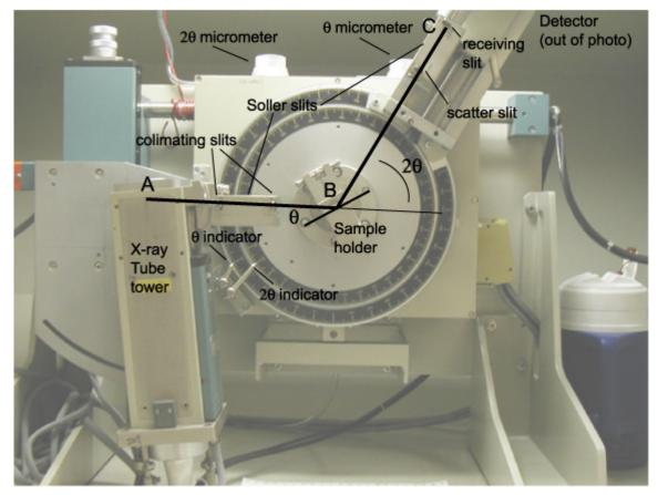
The photo above labels the important parts of our Scintag PAD V diffractometer. The following items are noted with differences between the Scintag and Brukker systems.
