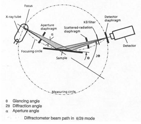
The diagram above is from the Siemens (now Brukker AXS) manual for the D5000 diffractometer. While placement and geometry is somewhat different between different systems, all the basic elements of a Bragg-Brentano diffractometer are present:
