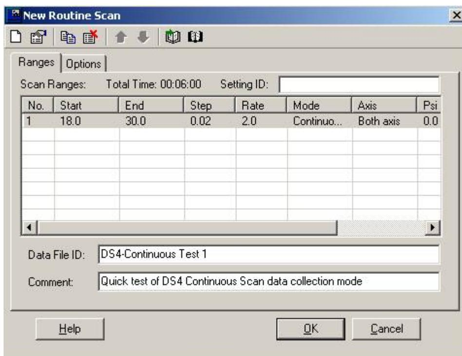
**Saving Scan Parameters:** The scan parameters may be saved to a separate file in your personal “Scan Book” by clicking on the save parameters icon (the open book icon with the arrow), so that the parameters may be reused for other scans. The open book (without the arrow) may be used to retrieve previously saved setups from your “Scan Book”.
