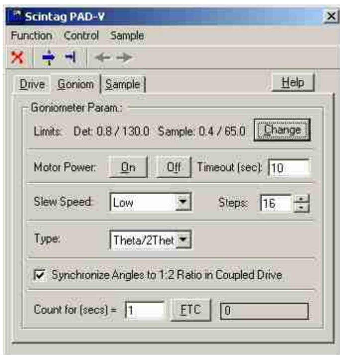
Again select the “Control” menu in the main DataScan Window and select “Databox” to bring up the “Scintag PAD-V” window shown at left.
