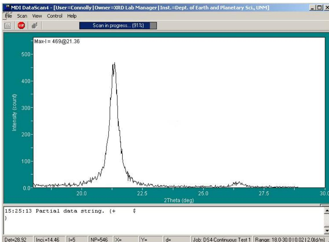
When data collection is done, the display written and the diffractometer is parked at the  $10^\circ 2\theta$  “exchange” position\*, exit the program (**File** menu – **Exit**). If you are finished using the system, log off the network to close your network connection.
