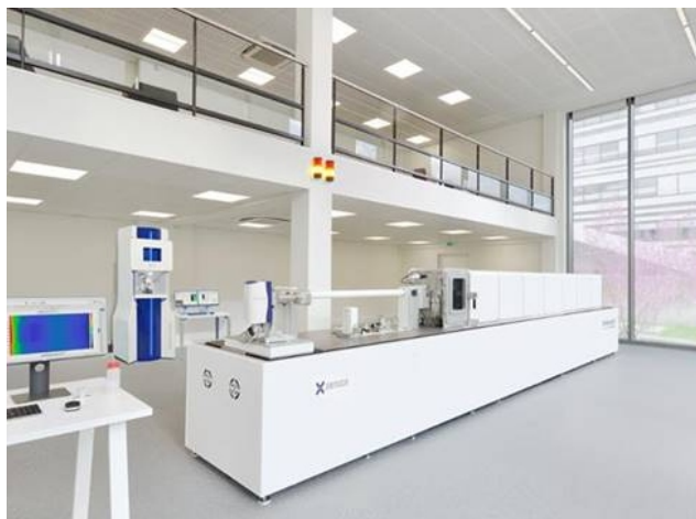
Figure 1. Xeuss Pro horizontal platform for SAXS/WAXS/GISAXS/USAXS and imaging alongside the Nano-inXider compact vertical system.
