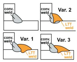
Figure 2. Cross section of the geometries.
