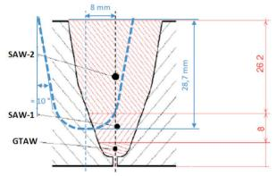
Figure 1. Schematic drawing of the original "U" groove and the repair excavation (dashed blue line).
