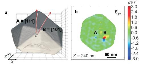
**Figure 1**. (a) Wireframe plots of the reconstructed electron density of a Pt particle drawn at 35% of the maximum density. A dislocation loop is evidenced. (b) Two-dimensional cut of the out-of-plane strain,  $\varepsilon_{zz}$ , at a particle height of 240 nm.
