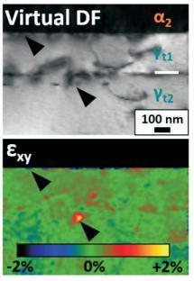
Figure 3. Recorded strain map of a lamellar structure.
