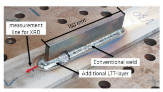
Figure 1. Longitudinal stiffener with additional LTT.
