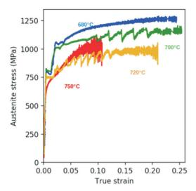
**Figure 3.** Comparison of Von Mises Stress in austenite for four intercritical temperatures.
