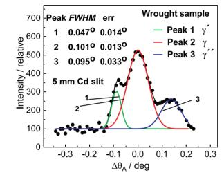
**Figure 4.** Analyser rocking curve rela-ted to the wrought Inconel 718 sample.
