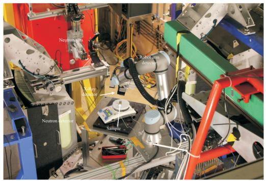
Figure 1. X-Raybot installed on ENGIN-X neutron instrument
