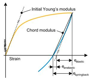
Figure 1 Schematic stress-strain curve to illustrate material behaviour and parameters.
