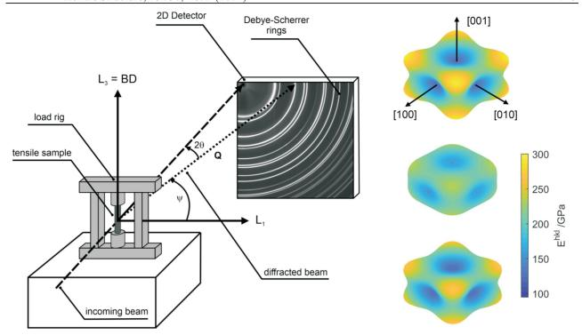
Figure 3. Determination of diffraction and single-crystal elastic constants [2].
