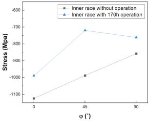
Figure 1. Residual stresses of inner-race bearing.
