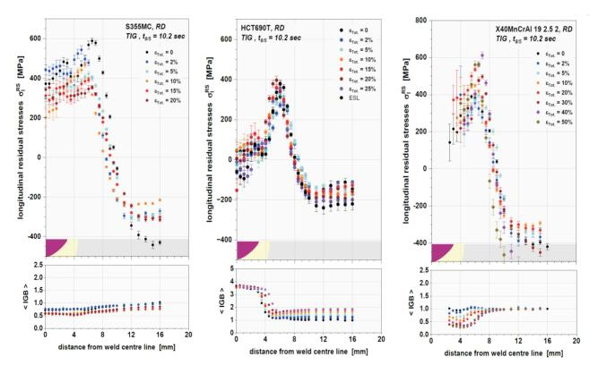
Figure 1. Comparison of the longitudinal residual stresses in different cold formed steels after TIG-welding.
