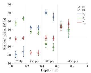
**Figure 2.** Measured residual stress distribution in a  $[0/45/90/-45]_s$  laminate.
