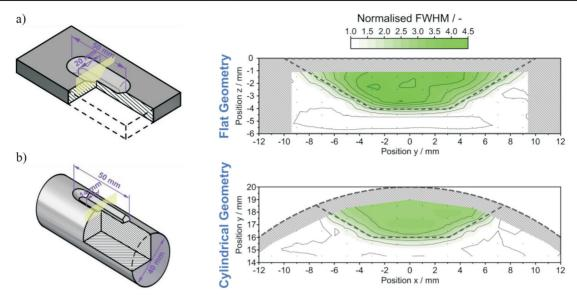
**Figure 1**. Schematic of the investigated flat (a) and cylindrical (b) geometries with a tapered cavity filled by means of cold gas repair spray. All dimensions given in mm.
