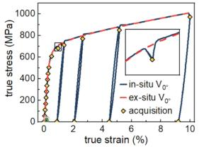
Figure 1. True stress-strain curve during in-situ loading [1].
