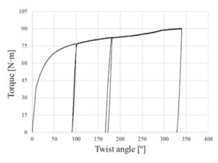
**Figure 1**. Torsion test in a steel sample (load-unload cycles at 100°, 180° and 340°).
