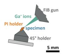
Figure 1. Sketch of specimen fabrication via FIB.
