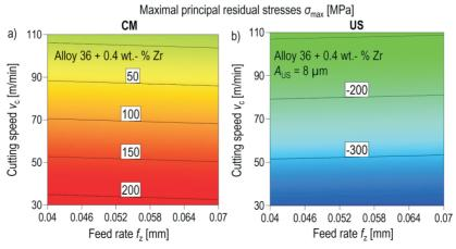
Figure 1. Maximal principal residual stresses  $\sigma_{\text{max}}$  versus cutting speed  $v_c$  and feed rate  $f_z$  for a) conventional milling and b) ultrasonic-assisted milling.
