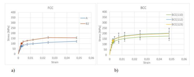
**Figure 2.** Resolved shear stress evolution during elastoplastic deformation versus sample strain E for slip systems in  $\alpha$  (a) and  $\beta$  (b) phases of CuZn39Pb3 brass.
