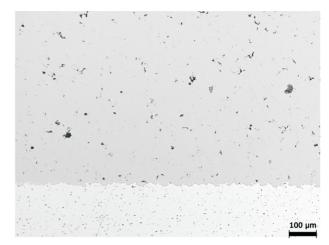
Figure 1. Typical microstructure of grade 1 Titanium coatings deposited on AlMg3 substrates.
