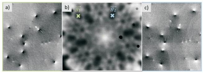
**Figure 1**. a) 15 keV electron channelling contrast image (ECCI) from a GaN specimen revealing threading dislocations, i.e. spots with black-white contrast. b) The specimen orientation is revealed from the electron channelling pattern (ECP)m where two diffraction conditions are identified (g1 & g2). Same defects are imaged a) and c) under these two diffraction conditions, showing contrast change that enable defect classification.
