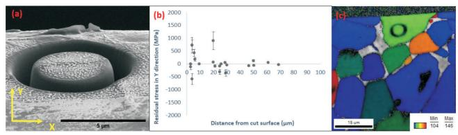
**Figure 1**. (a) FIB-DIC ring-core milling; (b) Residual stress values in the Y direction (perpendicular to the cut surface) versus distance from the cut surface; (c) Map obtained via EBSD after FIB-DIC milling, showing the local variation of Young's modulus (GPa) in the Y direction close to the cut surface.
