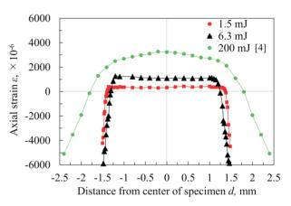
**Figure 1**. Axial strain distributions along the diameter axis of laser peened Ti-6Al-4Vround bar specimens measured at SPring-8/BL22XU.
