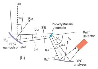
**Figure 1.** Schematic drawing of the 3-axis diffractometer setting using BPC monochromator and analyzer and a polycrystalline sample of a small width - (a), as well as the configuration of the setting for a sample of a rather large width - (b).
