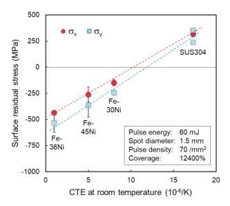
Figure 4. Relation between CTE and surface RS.
