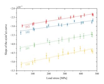
**Figure 1**. Measurement results after four-point bending to determine the X-ray elastic constants  $(1/2)S_2^{hkl}$  of WC-Co.
