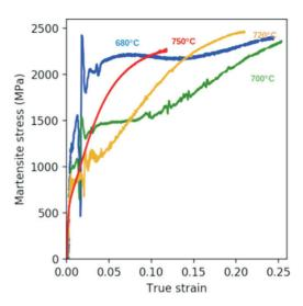
**Figure 4.** Comparison of Von Mises Stress in martensite for four intercritical temperatures,
