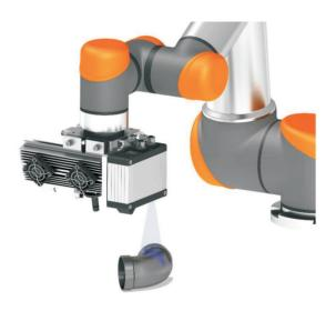
Figure 1. 3D scanner mounted on the X-Raybot.
