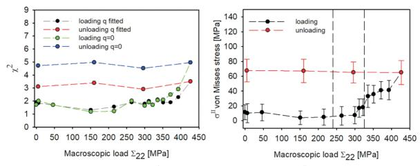
**Figure. 2.** Evolution of fitting quality parameter  $\chi^2$  and mean von Mises second order stress  $\sigma^{II}_{Mis}$  vs. macroscopic true stress  $\Sigma_{22}$ .
