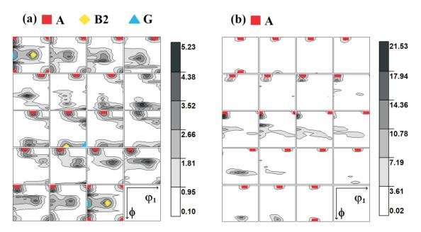
**Figure 1.** Orientation distribution function for the  $\alpha$  (a) and  $\beta$  (b) phases of CuZn39Pb3 brass. Cross-sections through the reduced space of Euler angles are shown, with the step of 5° along the  $\varphi_2$  axis.
