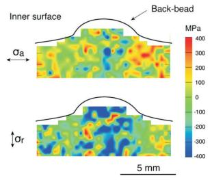
**Figure 2**. Residual stress maps around back-bead of welded pipe. The axial and radial stresses are obtained by combining the axial and radial strains measured by the DEM and the hoop stress measured by neutrons.
