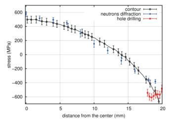
**Figure 1**. Ti-6Al-4V cylindrical specimen: a) Two-dimensional map of the axial residual stresses determined by the contour method in the median plane. b) Comparison between the axial residual stress profiles determined by the contour method (along the dashed line represented in a), by neutron diffraction and by hole drilling.
