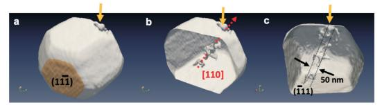
**Figure 2.** (a) 3D imaging of a 400 nm Pt nanocrystal during nanoindentation. (b) Dislocation network at the onset of plasticity (c) Identification of glide planes and dislocation loops size.
