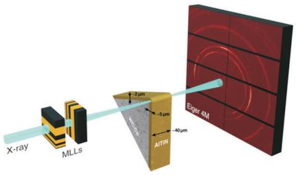
**Figure 1.** The CSnanoXRD setup in shows the cross-sectional lamellae prepared from a cutting insert, the sample is scanned in transmissional geometry. Multilayer Laue lenses enabled a beam size of 75×75 nm, on the sample, a step of 50 nm was used to map the thin film microstructure and stress at the cutting edge.
