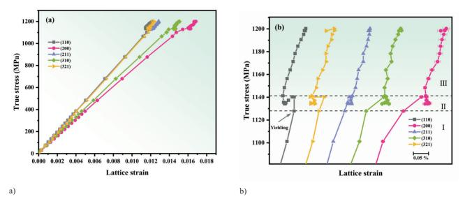
Figure 2. (a) True stress—lattice strain curves for five  $\frac{\sinh \sqrt{LD}}{\sinh \theta}$  families of grains obtained during tensile loading at room temperature. (b) Magnified lattice strain evolution with true stress for the  $\frac{TiZrHfNb}{98}N_2$  RHEA during yield and plastic deformation process.
