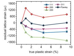
**Figure 2**. Residual strain accumulation of various lattice planes [1].
