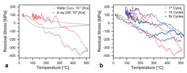
**Figure 1.** (a) Two stress-temperature diagrams are displayed which were measured at heating rates of 10<sup>-1</sup> and 10<sup>6</sup> K/s, by wafer curvature and XRD respectively. (b) Up to 5000 periodic heating cycles between 100-400°C were applied leading to a weakening of the Cu metallization due to fatigue.
