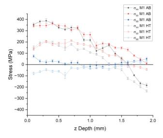
Figure 2a. Residual stress of the M1 part in the three principal directions both as built (AB) and after heat treatment (HT).
