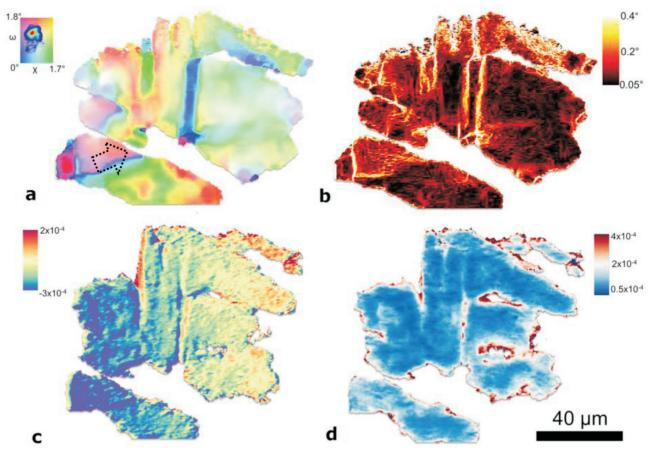
Figure 2. Reconstructed DFXM data from an as-deposited Cu thin film. Displayed are: (a) results from a mosaicity  $\omega$ – $\chi$  scan, (b) kernel average misorientation, (c) the  $2^{nd}$  order X-ray elastic strains and (d) the FWHM values in degrees [3].
