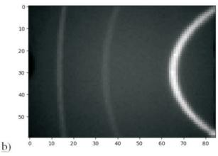
Figure 1. X-Solo device for residual stresses measurements (a) and diffraction rings observed for an iron powder (b).
