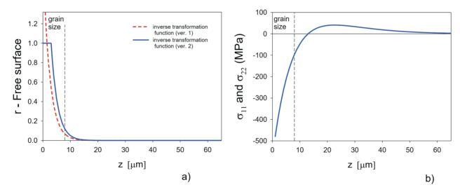
Fig. 1 The in-depth dependence of grain interaction (a), described by the r parameter (tunable free-surface model [4]) and stress  $\sigma_{11} \approx \sigma_{22}$  (b) in function of the real depth z below the surface. The results were obtained on the basis of different types of diffraction tests performed for mechanically polished austenitic sample.
