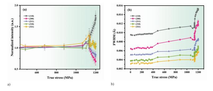
Figure 3. Evolution of diffraction peak intensity (a) and FWHM (b) of the  $(TiZrHfNb)_{98}N_2$  RHEA as a function of applied stress during tension.
