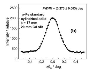
Figure 3. Examples of two analyser rocking curves for the  $\alpha$ -Fe(110) samples of  $\phi = 8$  mm - (a) and 17 mm - (b), respectively, both situated in horizontal position when simulating a large width of the irradiated gauge volume.
