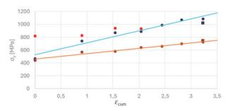
**Figure 1**. Example comparison of yield thresholds as a function of cumulative strain for conventional tension and compression tests; points corresponding to dynamic compression were also
