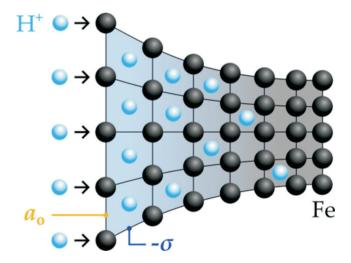
**Figure 1.** Illustration depicting the atomic lattice structure of a material subjected to electrolytic hydrogen charging, along with the ensuing gradients of lattice swelling and stresses between the free surface (left) and the bulk (right).
