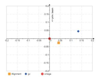
**Figure 1**. Positions of sample stage rotation centre (red), zero position of the alignment system (orange) and gauge volume position (blue) as determined by our alignment procedure. The scale is in mm.
