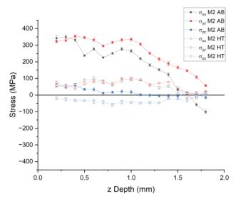
**Figure 2b.** Residual stress of the M2 part in the three principal directions both as built (AB) and after heat treatment (HT).
