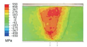
**Figure 2.** Residual hoop stress Contour map obtained on one of the weld repairs conducted on this project in the as-welded condition.
