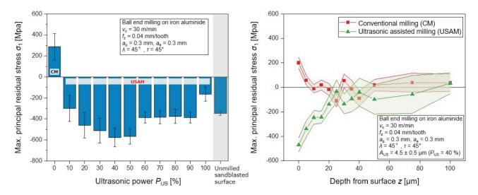
**Figure 2**. Maximal principal residual stresses  $\sigma_{max}$  under variation of the ultrasonic power  $P_{US}$ .
