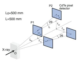
**Figure 1**. Double exposure method. The diffraction is measured by the area detector at P1 and P2.
