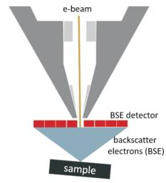
**Figure 1**. Schematics of Electron Channelling Contrast Imaging (ECCI) experimental setup performed in a SEM. Under specific specimen orientation the strain fields around threading dislocations are visualized by detection the backscattered electron using a BSE detector.
