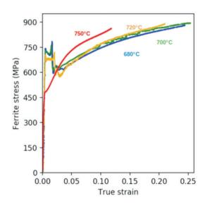
**Figure 2**: Comparison of Von Mises Stress in ferrite for four intercritical temperatures
