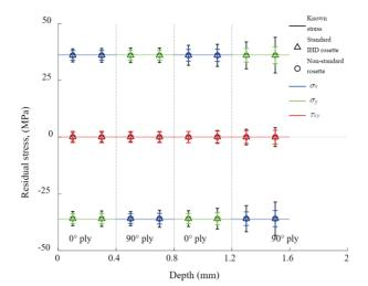
**Figure 1**. Measured residual stress distribution in a  $[0^{\circ}/90^{\circ}/0^{\circ}/90^{\circ}]_s$  laminate.
