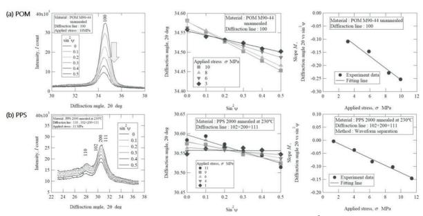
**Figure 1**. Measurement results of (a) POM and (b) PPS; Left is the diffraction peaks observed by  $\sin^2 \psi$  method, middle is the  $2\theta - \sin^2 \psi$  diagrams in each tensile load stress, and right is the M -  $\sigma_{app}$  diagram.
