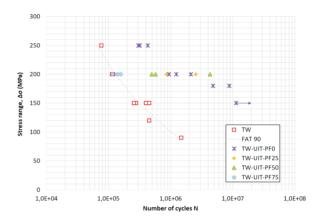
**Figure 1**. Fatigue life for each series of specimens.
