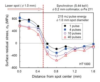
Figure 1. Surface RSs in and around laser spot.
