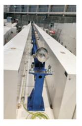
Figure 1. Left: Experimental area of BEER, CAD view from detailed design. Right: Installed neuron guides.
