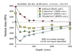
Figure 3. Overlap effect on RS of SUS304.
