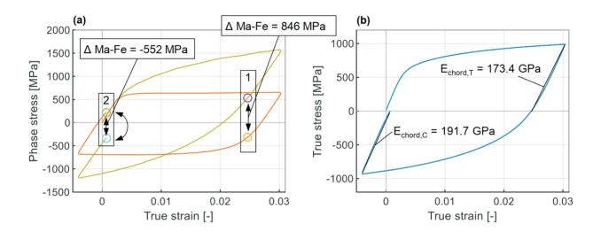
**Figure 3.** (a) Phase stresses and the interphase stresses at zero macroscopic stress after tensile loading (state 1) and after compressive loading (state 2) are plotted. b) True stress-strain curve and elastic chord moduli for tension Echord,T and compression Echord,C
