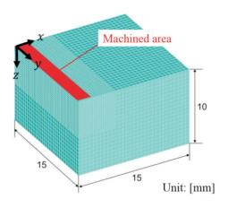
Figure 1. FE model used for numerical analysis.
