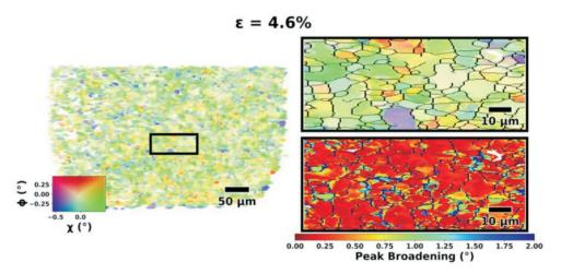
Figure 1. Orientation map with IPF colour code of aluminium sample deformed to  $\varepsilon = 0.046$ . Zoom in on region marked in on the left with misorientations above  $0.4^{\circ}$  as black lines. Corresponding peak broadening map, indicative of the local dislocation density and residual strain.
