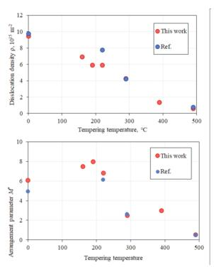
**Figure 1.** Obtained dislocation density (above) and arrangement parameter (bottom) via LPA as a function of tempering temperature
