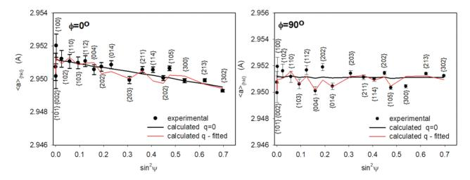
Figure. 1. Measured lattice parameters (points) and theoretical results (lines) vs.  $\sin^2 \psi$  for unloaded sample. Red lines for  $q \neq 0$  (the second order stresses are taken into account) and black lines for q=0 (the influence of second-order stresses is neglected).
