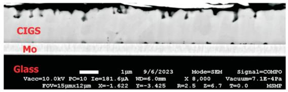
Figure 1. CIGS PV cross section, BSE SEM image.
