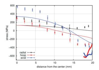
**Figure 2**. Residual stress radial profiles in Ti-6Al-4V sample median plane, determined experimentally from neutron diffraction (dots) and hole drilling method (bold lines). Calculated stress profiles (thin lines) obtained by numerical simulations. The latter show the average of stresses calculated in  $\alpha$  and  $\alpha$ ' phases.
