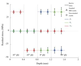
**Figure 2.** Measured residual stress distribution in a  $[+45^{\circ}/-45^{\circ}/0^{\circ}/90^{\circ}]_s$  laminate.
