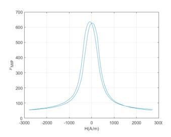
Figure 1. a) MIP Illustration and definition of MIP and b) example of incremental permeability measurement.
