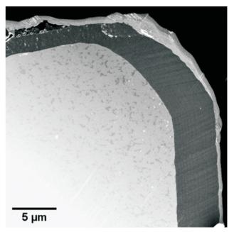
**Figure 2.** SEM micrograph of a FIB-prepared cross-section of the cutting edge reveals substantial differences in the thin film microstructure at the curved and planar substrate regions, respectively
