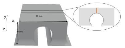
**Figure 1**. LPBF additively manufactured arch geometry and cross section view showing measurement path at the centre of the part in orange.
