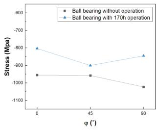
Figure 2. Residual stresses of ball bearing.
