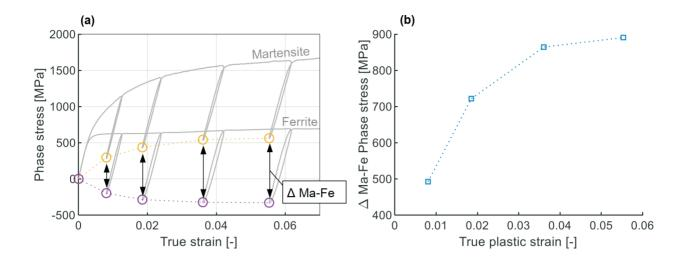
**Figure 2.** (a) Phase stress versus true strain. Highlighted are the phase stress at unloaded state (0 MPa) and their difference (delta). (b) Delta values at unloaded state versus true plastic strain.
