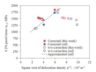
**Figure 2.** 0.2% proof stress obtained by tensile test as a function of the square root of dislocation density. Results in the past work [4] and this work were agreed. The corrected plots in both the past and this work were aligned on the approximated line.
