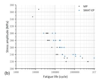
Figure 1. S-N plot for (a) MP and SMATed specimens, and (b) MP and SMAT-EP specimens.
