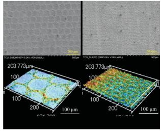
**Figure 2.** SEM (upper) and laser microscope (lower) images of Ti-6Al-4V treated by the low-energy LPwC with laser energy of 1.5 mJ.
