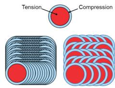
Figure 2. Overlap effect of laser pulses on RS.
