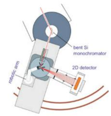
Figure 1. The layout of the HK4 strain scanner [1]
