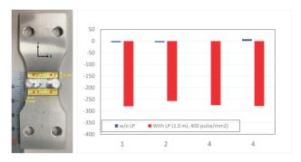
Figure 1. Surface Residual stress of A5083 welded sample
