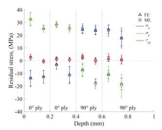
**Figure 1**. Measured residual stress distribution in a [0/0/90/90], laminate.
