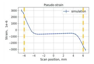
**Figure 2**. A simulated pseudo-strain distribution (sample surface is marked with yellow dashed line). The PS magnitude and distribution depends on the actual sample geometry, material and experiment geometry.
