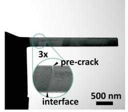
Figure 2. Finished cantilever in STEM mode.
