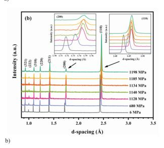
**Figure 1.** (a) True tensile stress-strain curve for tensile loading of the (TiZrHfNb) $_{98}N_2$  RHEA, the inset in (a) shows the work-hardening rate curve of the current RHEA. (b) Selected neutron diffraction patterns collected with respect to the loading direction during tensile loading of (TiZrHfNb) $_{98}N_2$  RHEA.
