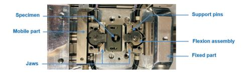
Figure 2. In situ SEM bending test setup.
