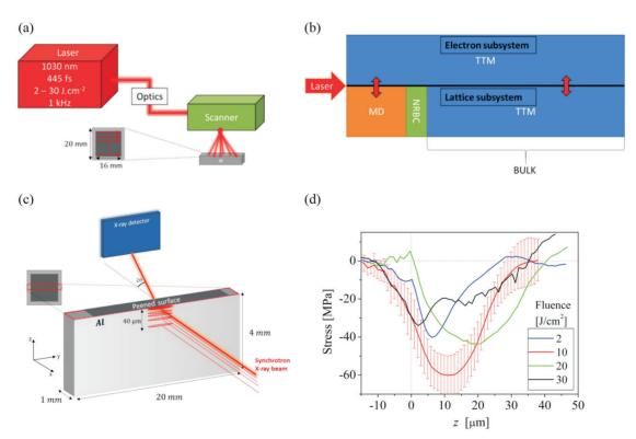
**Figure 1**. Schematic drawing of (a) the experimental setup of laser peening, (b) the geometry of numerical simulations, (c) and the synchrotron X-ray measurements. (d) Evolution of the measured residual stresses below the irradiated surface for various incident fluences.
