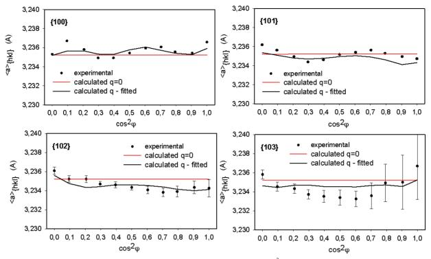
Figure 2. Measured lattice parameters (points) and theoretical results (lines) vs.  $\sin^2 \psi$  for unloaded sample. Black lines for  $q \neq 0$  (the second order stresses are taken into account) and red lines for q = 0 (the influence of second-order stresses is neglected).
