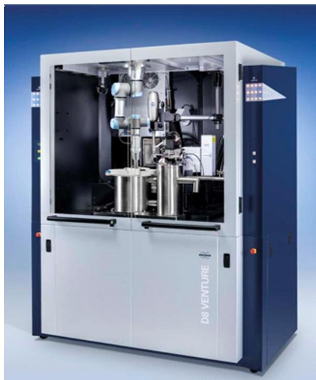
**Figure 1.** The D8 VENTURE system for macromolecular crystallography.
