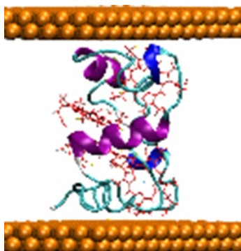
Figure 1. (a) DFT model of STC junction between gold electrodes. (b) Predicted current magnitudes using incoherent hopping and coherent tunneling models under resonant and off-resonant conditions.
