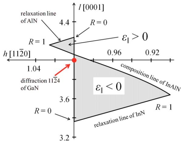
**Figure 1.** Schematic drawing of the admissible positions of the 1124 diffraction spot of InAlN layer for various composition  $x$  and degree of relaxation  $0 < R < 1$ . Note the sign of the in-plane strain component  $\epsilon_{||}$  is opposite in Al rich and In rich regions. For the sake of clarity the width of the area is 6-times enlarged.
