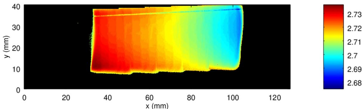
Figure 3. Map of 311 diffraction peak position measured at bent silicon wafer.
