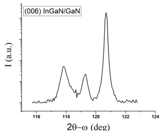
Figure 2. Diffractogram showing the (006) InGaN and GaN reflections and a hybrid peak
