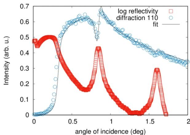
Figure 2. Angle of incidence dependence of FeCo 110 diffraction signal. Reflectivity curve in logarithmic scale.
