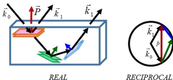
Figure 1. Geometry of a three-beam MD in real and reciprocal space.
