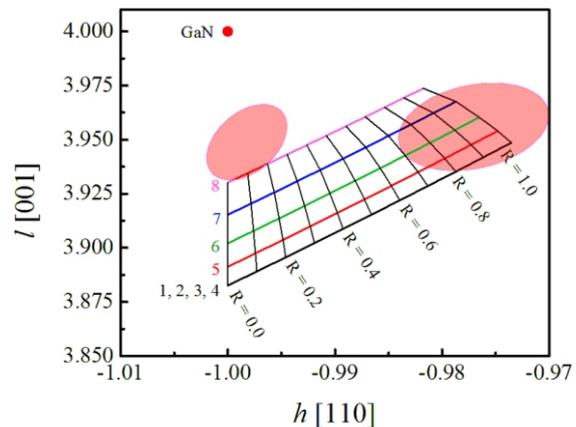
**Figure 3.** Composition & Relaxation diagram of InAlGaN layer. The position of two maxima revealed by X-ray RSM are schematically shown as ellipses.
