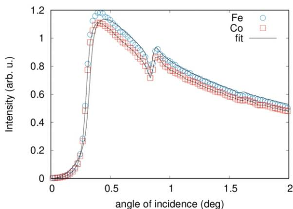
Figure 1. Angle of incidence dependence of Fe and Co fluorescence signal.
