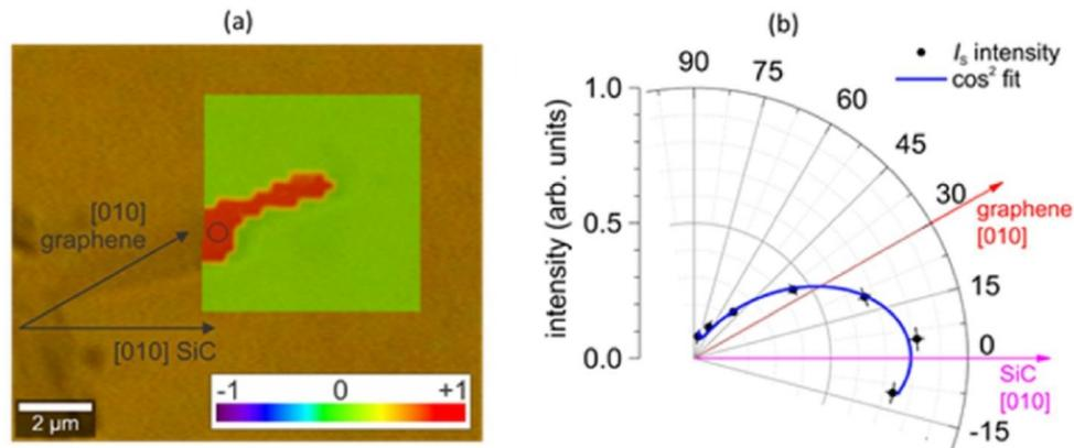
**Figure 3.** (a) Overlap of the optical and Raman images of a PEN island and (b)  $\cos^2$  fit of the azimuthal dependence of Raman band integral intensity at  $1373\text{ cm}^{-1}$  (short molecular axis vibrations) inside the black circle in (a).
