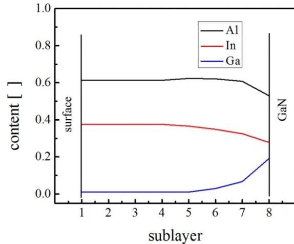
**Figure 2.** Depth profile of InAlGaN layer composition. The distance between the adjacent sublayers is  $\sim 40$  nm.
