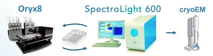
The Oryx8 in combination with the SpectroLight 600 can identify promising conditions for structure determination by cryoEM (and crystallization).
