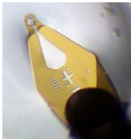
Crystal Mounting using MiTeGen's MicroMounts™.
