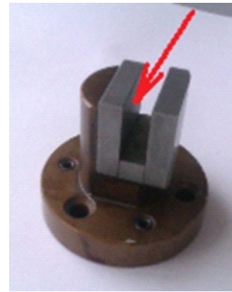
Figure 4. “Artificial” Ge channel-cut monochromator (assembled, glued together). Red arrow shows machined inner diffraction surface of the channel-cut monochromator glued to the metal block.
