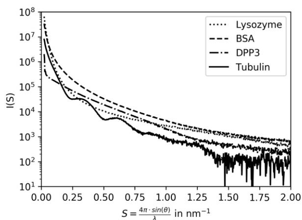
**Figure 2.** SAXS profiles recorded at the P12 BioSAXS beamline at the EMBL outstation in Hamburg, Germany. Tests of the flow cell with lysozyme, bovine serum albumin and human dipeptidyl peptidase 3 (DPP3) are shown alongside the scattering of Taxol-stabilized microtubules.
