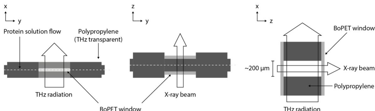
**Figure 1.** Design sketch of the THz- and X-ray-compatible flow cell. The chamber prototype is made of 3D-printed, THz-transparent polypropylene with windows made of biaxially-oriented polyethylene terephthalate (BoPET) for X-ray transmission.
