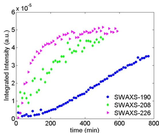
**Figure 2.** Evolution of the integrated 112 reflection of the S phase precipitate peak intensity at  $d = 2.570$  Å (or  $q = 2.445$  Å<sup>-1</sup>) at 190 °C, 208 °C, and 226 °C,...
