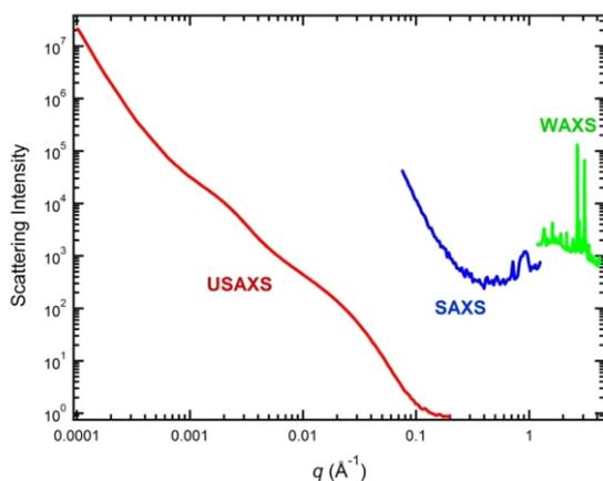
**Figure 1** Example of combined USAXS, SAXS, and WAXS for AA2024 alloy.
