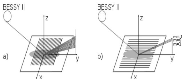
**Figure 1.** SAW experiment in meridional a) and sagittal b) geometry.
