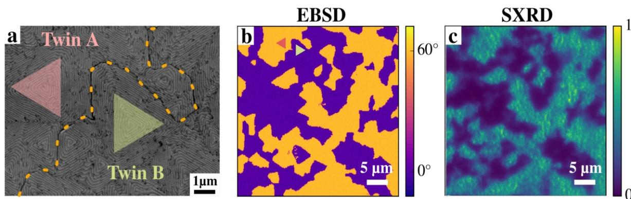
**Figure 1.** Twin formation in  $\text{Bi}_2\text{Te}_3$  thin films. a) Scanning electron micrograph of a twin boundary (dashed line) separating two crystallographically twinned areas. b) Electron backscatter diffraction (EBSD) inplane orientation map showing the twin domains in a larger area. c) bulk sensitive scanning XRD measurement of the very same area shown in b), however, with bulk sensitivity.
