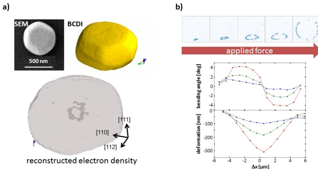
**Figure 1.** a) SEM image, reconstructed shape and electron density of an indented Au nanocrystal. b) Integrated diffraction patterns of the Au 222 Laue spot recorded along the deformed nanowire, bending angle and nanowire profile inferred from the diffraction patterns.
