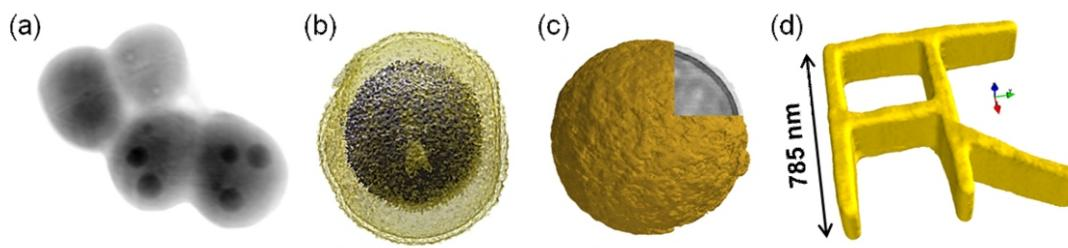
**Figure 1.** Reconstructed images: (a) *Deinococcus radiodurans* bacteria; (b) Vaterite core-shell particle (semitransparent iso-surface rendering); (c) Polymer microspheres with 3 coating layers (shown in a cut); (d) Tiny gold test sample. The scale bars are 1  $\mu$ m.
