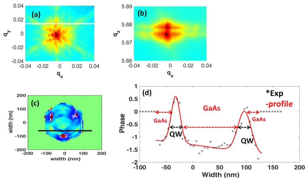
**Figure 1.** (a,b) Projections of the experimentally recorded 3D CXDI pattern from single NW around the GaAs (333) reflection.(c) Retrieved phase pattern of the nanowire. (d) Line cut from the phase shown in (c) black line.
