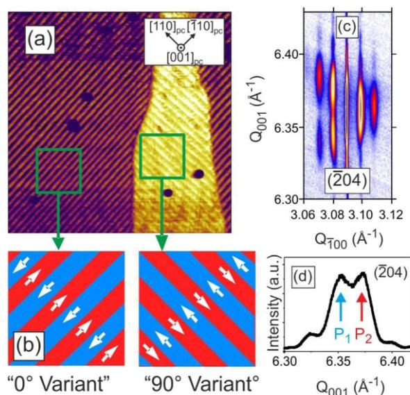
**Figure 1.** (a) Lateral PFM image ( $2 \mu\text{m} \times 2 \mu\text{m}$ ) of a 30 nm  $\text{K}_{0.75}\text{Na}_{0.25}\text{NbO}_3$  film grown on (110)  $\text{TbScO}_3$ , (b) models of  $0^\circ$  and  $90^\circ$  variants (white arrows indicate the in-plane component of the polarization vector), (c) out-of-plane x-ray diffraction and, (d) section along the CTR at  $Q_{-100} = 3.09 \text{ \AA}^{-1}$  (adapted from [1]).
