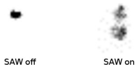
Figure 2. Bragg peak recorded with a CCD camera. When SAW are switched on the 0-th order is suppressed and the satellite peaks appear
