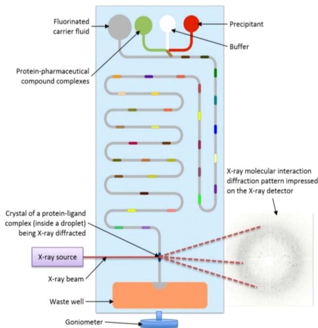
**Figure 1.** PharmaLab Card and XRD (concept)
