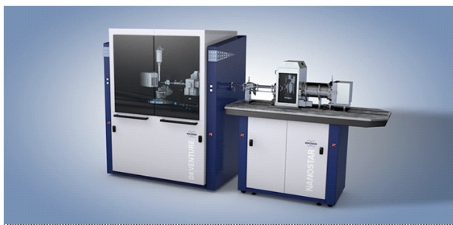
Figure 1. D8 VENTURE with NANOSTAR: Complete Home-Lab System for macromolecular crystallography and bio-SAXS.
