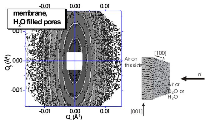
**Figure 2.** 2D cross-section  $d/d(Q_x, Q_y)$  is shown (left) for H<sub>2</sub>O filled pores of the porous membrane (scheme shown on right). The grey scale map shows measured 2D data and the white equi-intensity lines depict the fitted curves. V4 pinhole SANS, BENSC, HZ Berlin.
