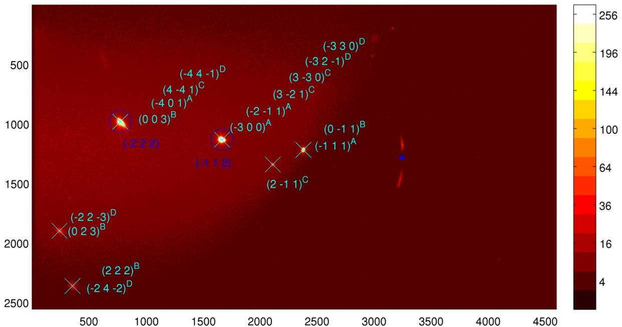
**Figure 5.** Possible indexing of an image taken in the oscillation mode. Intensity maxima can be indexed by (bcc) beta-Ti matrix (blue circles) and by 4 families (subindexes A, B, C, D) [5] of (hexagonal) omega-Ti (cyan crosses).
