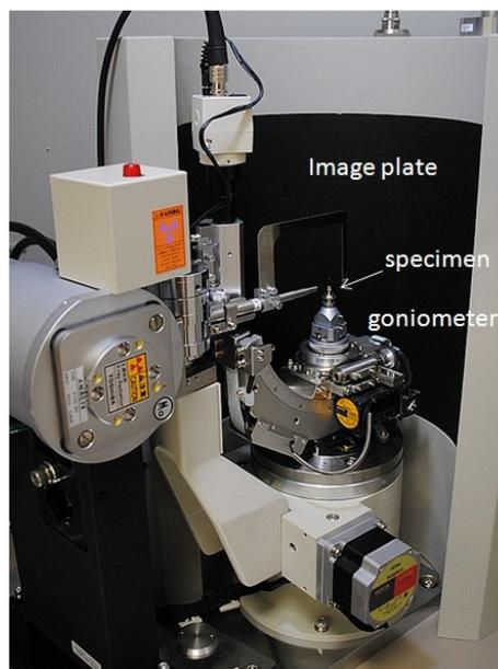
**Figure 1.** Rigaku R-Axis Rapid II diffractometer with image plate system.
