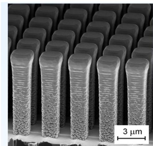
**Figure 1.** SEM image of epitaxially grown Ge crystals on etched 8  $\mu\text{m}$  Si pillars shows 1.2  $\mu\text{m}$  high crystals having pillar period 3  $\mu\text{m}$  and 1  $\mu\text{m}$  large trench.
