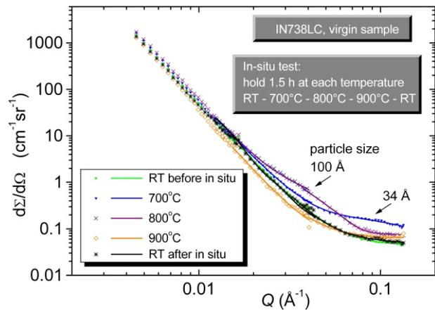
**Figure 1.** In-situ SANS for non-cycled sample: in-situ heating RT-700-800-900°C-RT (hold at each temperature during the in-situ SANS was always 1.5 hour).
