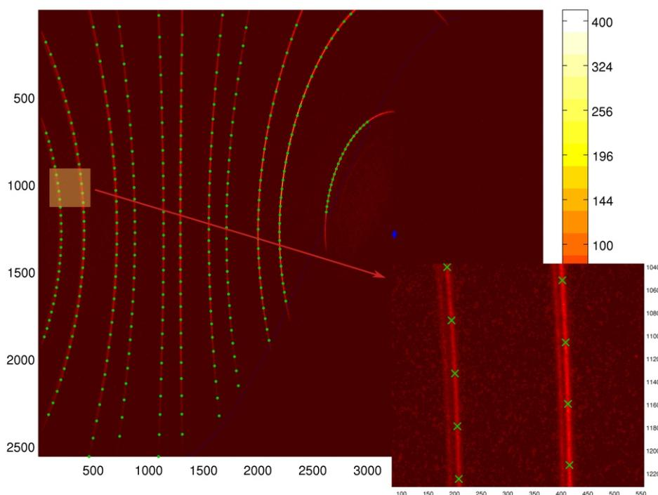
**Figure 3.** Analysis of Debye rings from the NIST standard Si powder sample for calibration of beam and sample displacement instrumental corrections. Diffracted intensity in the bottom right corner of the IP is shadowed by the goniometer head.
