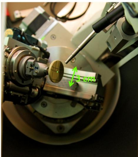
**Figure 2.** Florescent target mounted in the sample position. During a typical experiment two goniometer axes are set to fixed positions ( $\omega = 210^\circ$ ,  $\psi = 55^\circ$ ) and the sample is spinning/oscillating around the axis ( $\phi$ ) perpendicular to the sample surface.
