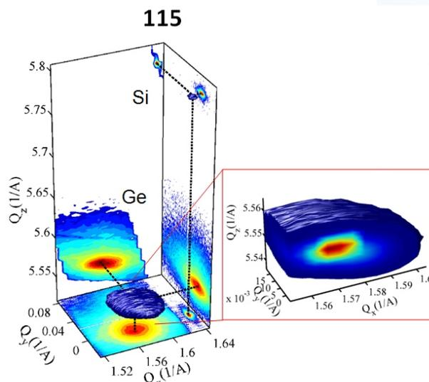
**Figure 3.** Example of 3D reciprocal space map recorded in the middle of the 3.1  $\mu\text{m}$  pillar showing detailed cut through Ge diffraction peak.
