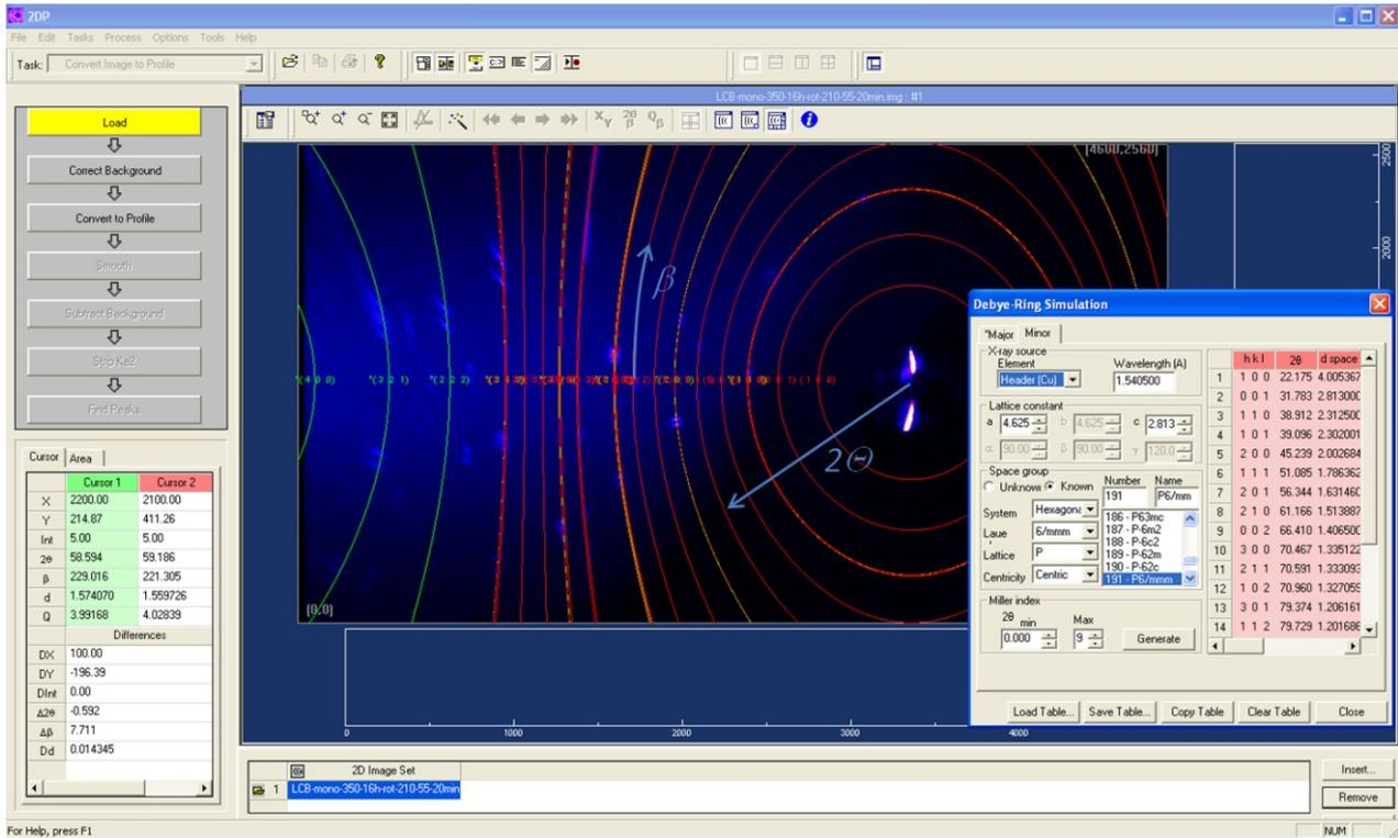
**Figure 4.** A preliminary analysis of the quick “survey” measurement of the LCB beta-Ti alloy single crystal using the Rigaku 2DP software. Simulated green Debye rings are related to the (bcc) beta-Ti matrix phase. Contrary red lines come from the minor omega-Ti nanoparticles. The lattices of both phases are coherent hence some beta-Ti green rings are overlapped with red rings of (hexagonal) omega-Ti.
