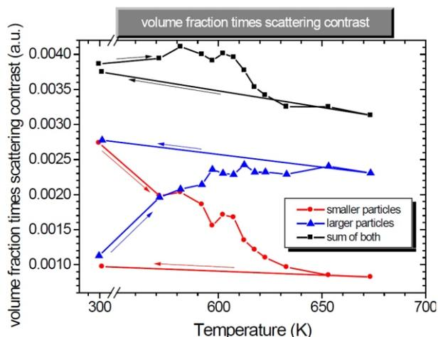
**Figure 3.** The temperature dependence of volume fraction times scattering contrast of confined Pb particles in the Al-4%Pb ECAP sample during the thermal cycle.
