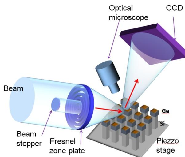
**Figure 2.** Experimental setup of scanning nanodiffraction experiment.
