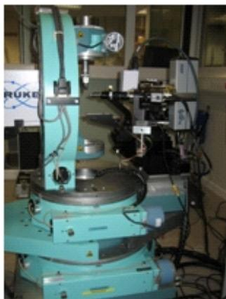
**Figure 2.** Upgrade of a Huber goniometer with a Ag,  $\text{I}\mu\text{S}$ .
