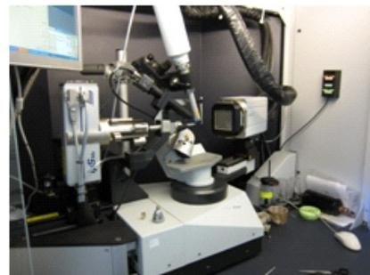
**Figure 3.** Replacement of a Mo sealed tube with a Mo  $\text{I}\mu\text{S}$  on a Bruker AXS X8.
