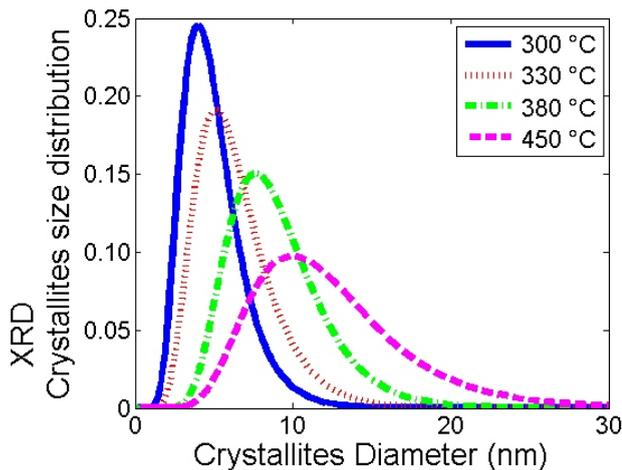
**Figure 5.** Crystallites size distribution of anatase nanopowders prepared from a same precursor and calcinated at different temper-
