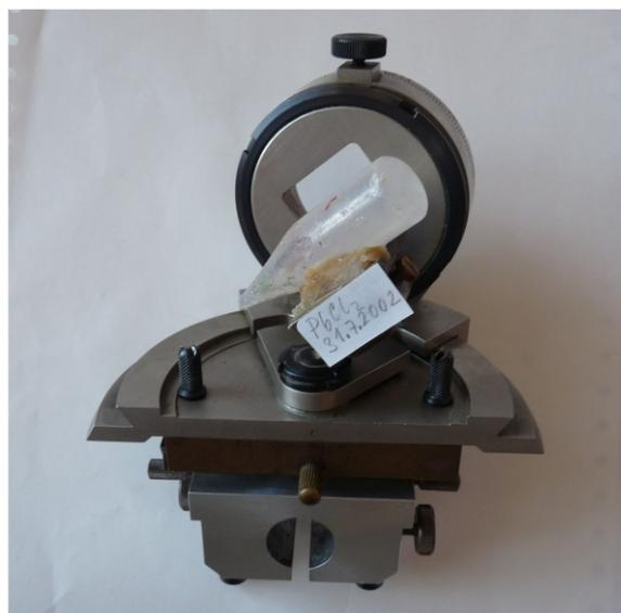
**Figure 2.** Crystal holder with Eulerian geometry.
