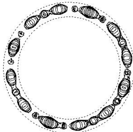
Figure 3. Pole figure (103) of YBaCuO layer grown on MgO buffer layer deposited on GaN/sapphire substrate. The range of angle is 40 – 50°.
