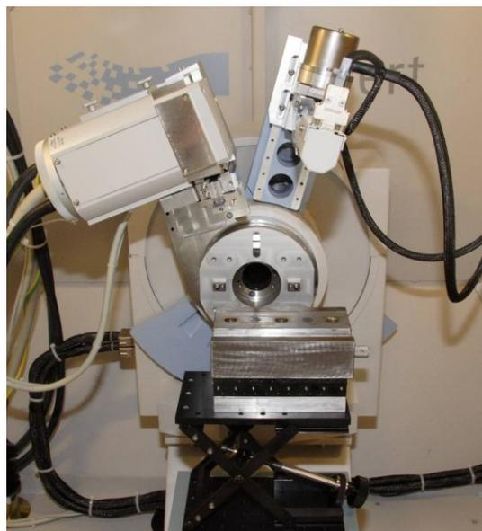
**Figure 1.** Mounting of a guide gib for residual stress measurement by X'Pert PRO.
