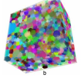
**Figure 1** (a) 3D phase map of an Al-Si alloy highlighting the Iron-rich inclusion (dark/red) between the Si particles (light/yellow). The image is acquired in divergent beam setup, the resulting effective voxel size is 50 nm. (b) Labeled individual bubbles of a rapidly evolving liquid foam. The whole volume of 2048 1024 pixels scanned in fast tomography mode with scanning time of 25 s, on the figure we show a region of 700 700 300 at pixel size 7.5 microns.
