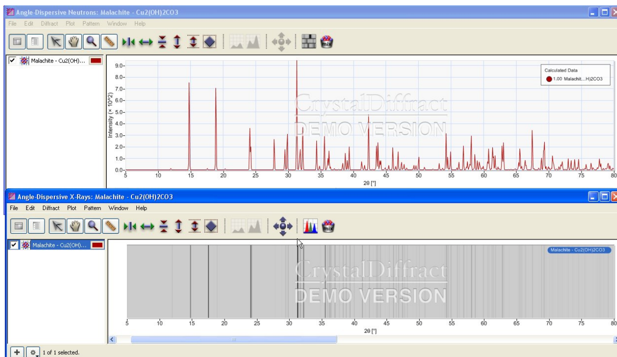
Figure 7. Two windows of CrystalDiffract - simulation of powder diffraction pattern obtained by the detector (top) and film record (bottom).
