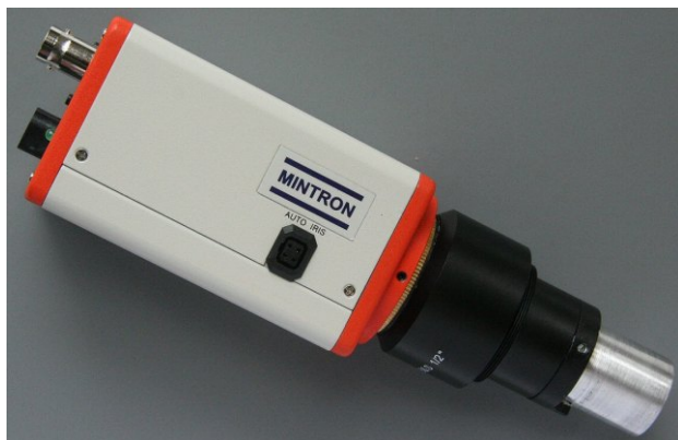
Figure 1. Mintron MTV-62W1P camera equipped with an optical interface.
