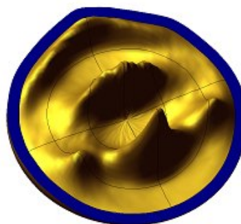
Figure 2. Pole figure (111) of 1 pass ECAP deformed Cu sample in classical contour plot (top) and the so-called 2.5 D plot (bottom).
