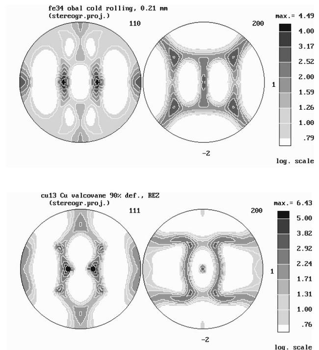
**Fig. 16.** An example of the pole figures of a tin plate steel (a) and a cold rolled Cu with 90% reduction [82].
