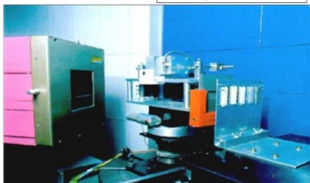
**Fig. 7.** Schematic diagram of the high resolution double-bent-crystal SANS diffractometer with the fully asymmetric diffraction geometry of the analyzer crystal in combination with a position sensitive detector and the photo of the sample and analyzer part.
