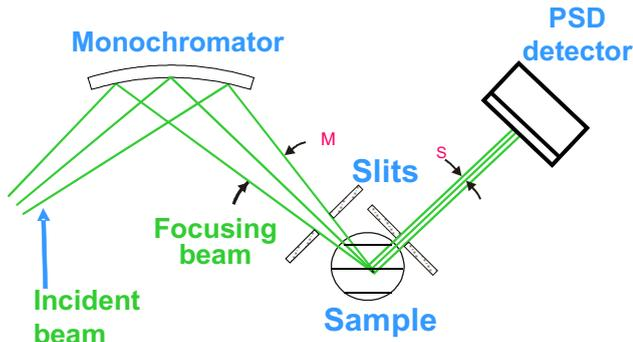
**Fig. 14.** Sketch of the focusing performance of the diffractometer dedicated to residual strain scanning [119].
