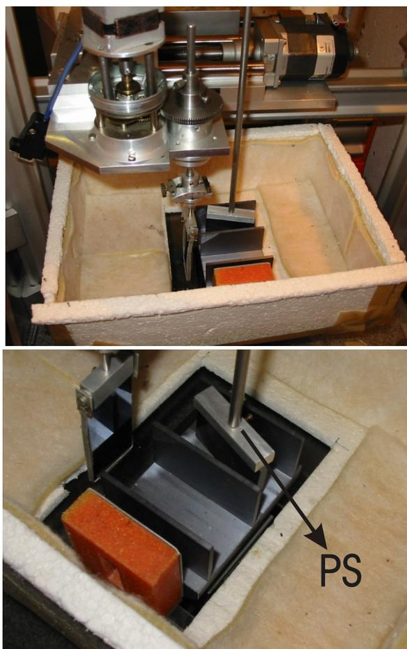
**Fig. 8.** The view of the three crystal interferometer of the type LLL with the phase shifter PS and the sample S arranged for the nondispersive measurement.
