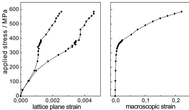
**Fig. 15.** Stress-strain dependences of related to the individual phases -111 and -110 of a duplex steel obtained from the diffraction experiment (left) as compared with the mechanical one (right).
