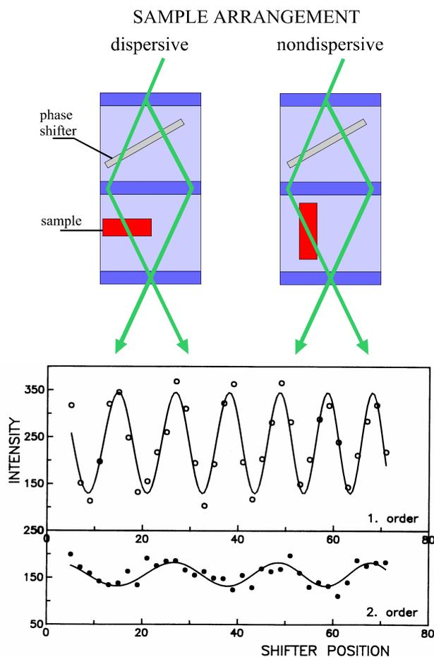
**Fig. 9.** Schematic diagram of the dispersive and nondispersive sample arrangement and the interference patterns observed in the O-beam of the interferometer simultaneously in the first- (220) and second-order (440) reflection by the TOF method at the pulsed neutron source.
