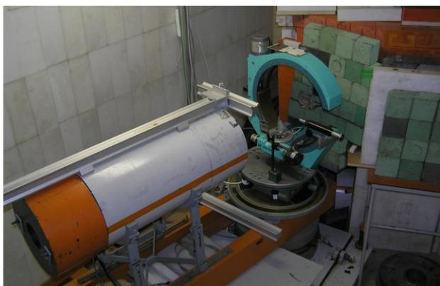
Fig. 10. Diffractometer for texture measurements moved from ZfK Rossendorf to NPI.
