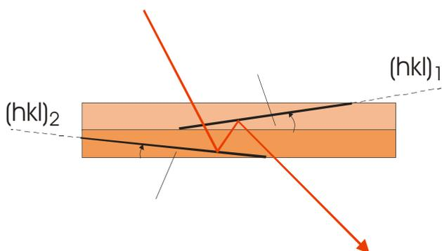
Fig. 12. Dispersive sandwich monochromator consisting of two bent perfect Si- slabs of different cut [128].
