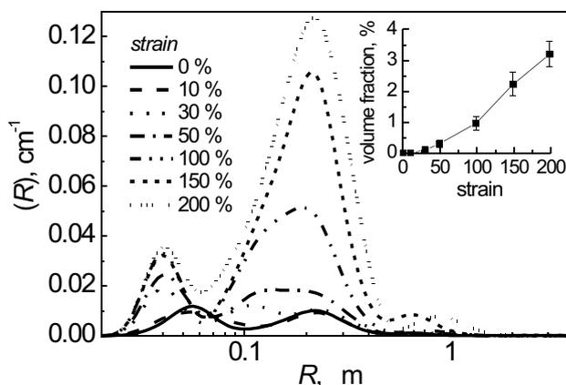
Fig. 13. Size distributions and integrated volume fractions of pores created in the course of super-plastic deformation of Y-TZP ceramics, as results from double-crystal SANS measurements [140].
