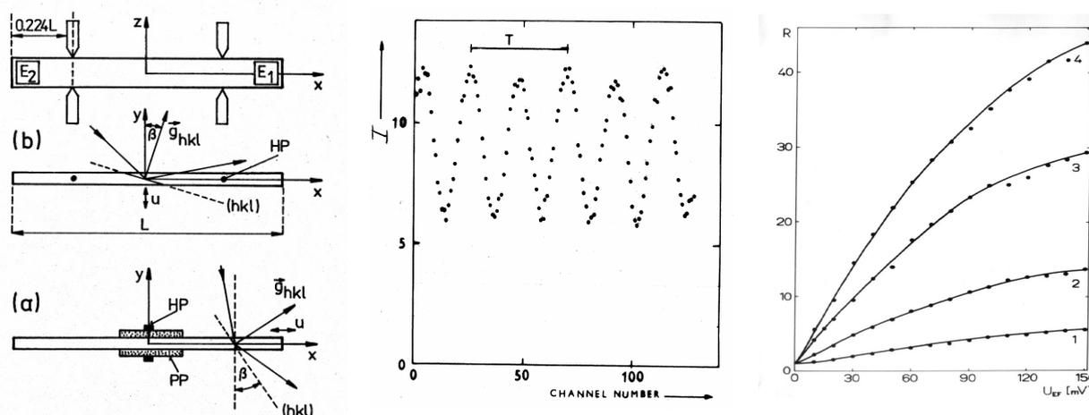
**Fig. 3.** Schematic sketch of performance for longitudinal crystal vibrations with the holding point at the nodal line in the middle (a) and flexural vibrations with two holding points (b), time modulation of the beam diffracted by longitudinally vibrating quartz single crystal and the relative increase of the integrated reflectivity dependent on the vibration amplitude for different thicknesses of the crystal (3 and 14 mm) and different wavelengths (0.105 and 0.154 nm) [8-11].
