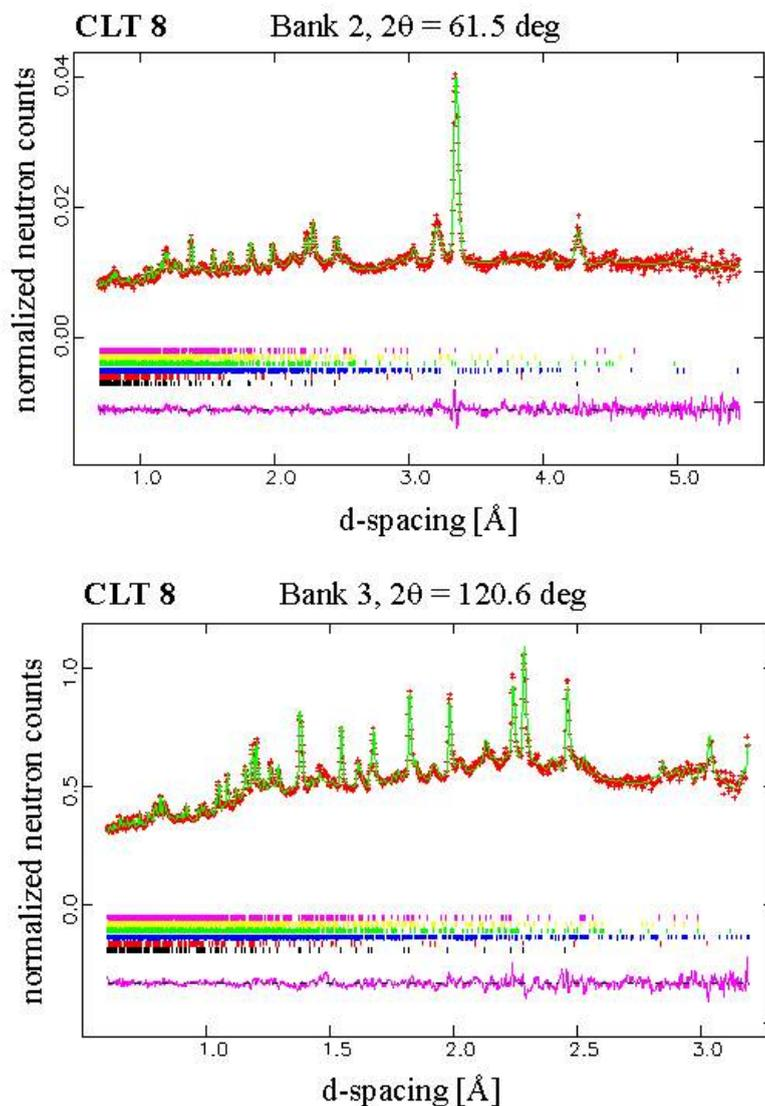
**Fig. 2.** Measured data (symbols), calculated pattern (solid line), and difference between the observed and calculated intensities (lower curve) of pottery sample CLT 8. The bar codes indicate the theoretical peak positions of the different phases (bottom to top): quartz, calcite, plagioclase, illite/muscovite, k-feldspar, diopside. The two patterns correspond to the forward (top) and backscattering detectors on ROTAX, respectively.
