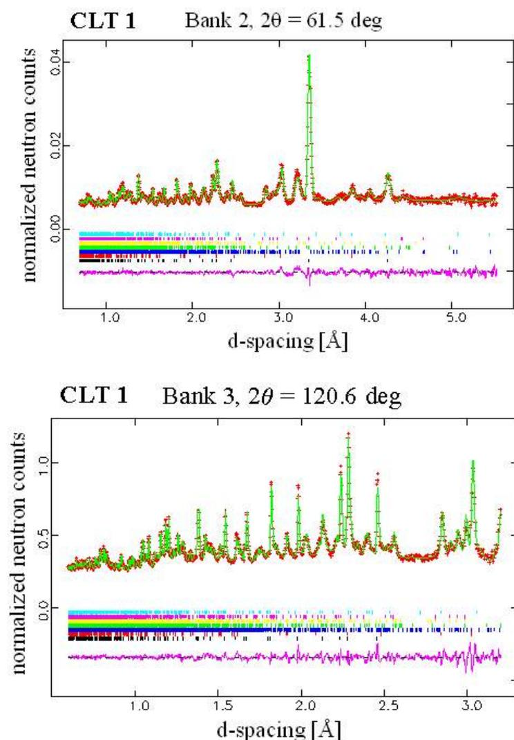
**Fig. 1.** Measured data (symbols), calculated pattern (solid line), and difference between the observed and calculated intensities (lower curve) of pottery sample CLT 1. The bar codes indicate the theoretical peak positions of the different phases (bottom to top): quartz, calcite, plagioclase, illite/muscovite, k-feldspar, diopside, gehlenite. The two patterns correspond to the forward (top) and back-scattering detectors on ROTAX, respectively.
