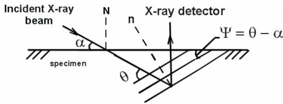
**Fig. 2.** Schematic of GIABD geometry;  $N$  and  $n$  – normals to the surface and to crystallographic planes.
