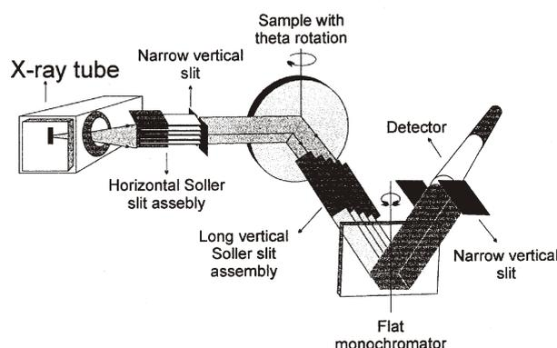
Fig. 1. Setup of URD-6 diffractometer for GIABD analysis.
