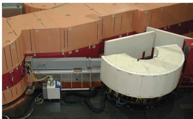
**Fig. 1:** Set-up of the Structure Powder Diffractometer SPODI at the FRM-II.
