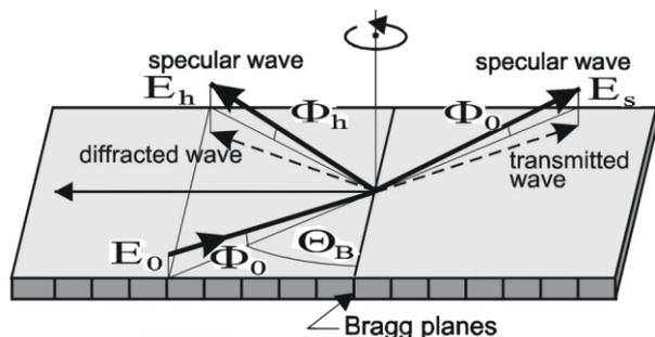
**Fig. 1.** Geometry of grazing incidence diffraction. (taken from [14]).  $E_0$  ... incident beam,  $E_s$  ... specularly reflected beam,  $E_h$  ... diffracted-reflected beam.
