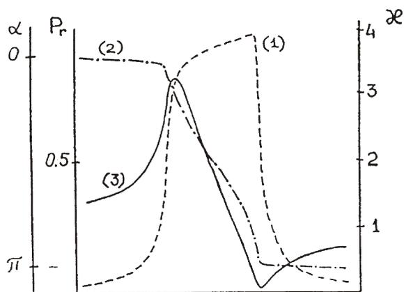
**Fig. 3.** Schematic picture of the angular dependence (  $\theta$  ) of the reflection coefficient (reflection curve) - 1 ( $P_R$ ), phase - 2 ( $\phi$ ) and the intensity of the wavefield at the atomic planes - 3 ( $I$ ) around the diffraction position [16].
