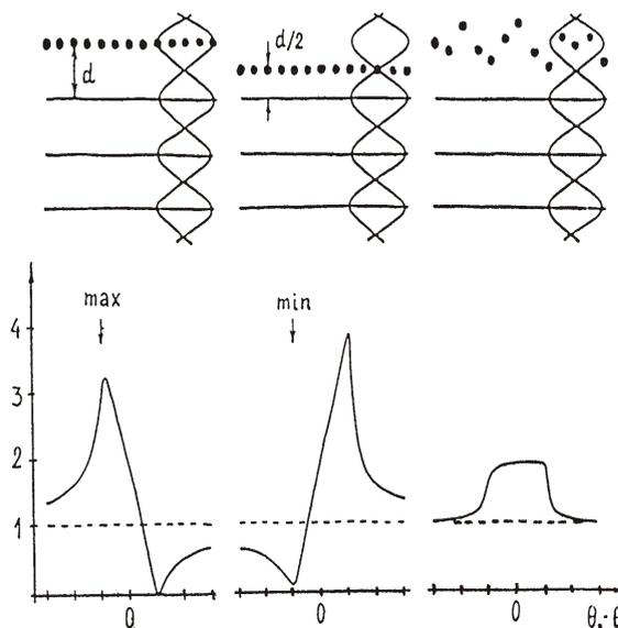
**Fig. 4.** Illustration of different positions of adsorbed atoms with respect to the antinodes of the XSW field and the corresponding yield of fluorescent radiation of the adsorbed atoms.
