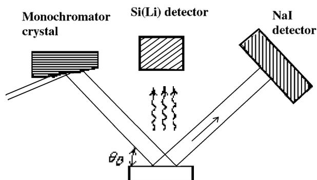
Fig. 5. Experimental arrangement for XSW measurement
