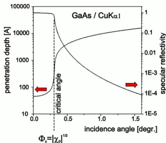
**Fig. 2.** Penetration depth and reflectivity curve at grazing incidence [14]
