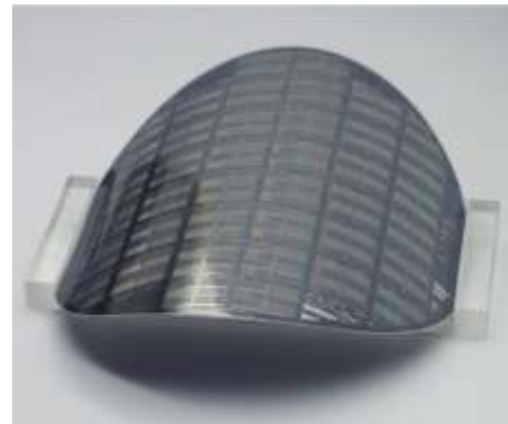
Fig. 1. Ultra-thin silicon wafers become mechanically flexible.
