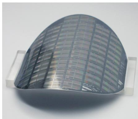
Fig. 1. Ultra-thin silicon wafers become mechanically flexible.
