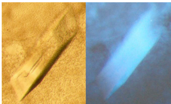
Figure 1. The single crystal of ST50 was illuminated under the white light (left) and the UV light (right).
